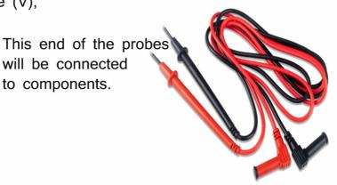
This end of the probes are attached to the Ports of the DMM.
